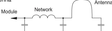
**Notice:** Do not install any ground surfaces or wiring under the antenna. Distance top side to ground or other potentials >5 mm.
