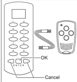
2. Keep button 2 on the Multi Channel Transmitter pressed until the memorizing symbol flashes in the display.
