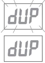
3. Within 10 seconds press the button of the source transmitter briefly and then the middle ENTER-button. You can release the ENTER- button of the target transmitter now.
