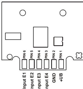
So it is possible to send 15 different telegramms, depending on the wiring of the inputs.
