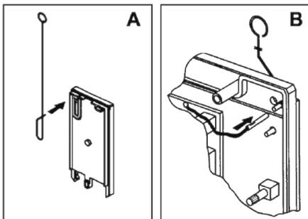
5. Connect the rod antenna (Fig. A).
