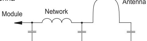
Notice: Do not install any ground surfaces or wiring under the antenna. Distance top side to ground or other potentials >5 mm.
