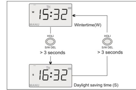
In this case, the clock is set back/forward by one hour.
