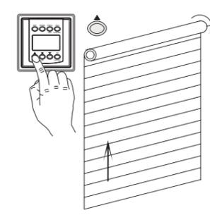
The tubular motor rotates in both directions for 1 second each.
