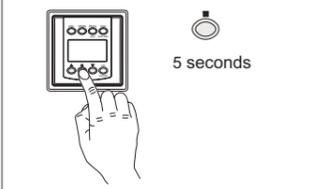
The tubular motor rotates in both directions for 1 second each.
