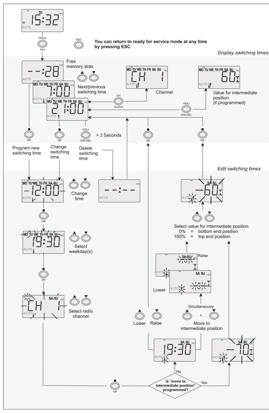
If move to intermediate position is programmed, the shutter/awning first moves to an end position and then to the desired intermediate position.
