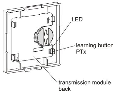
3. Re-insert the transmission group into the mounting frame.
