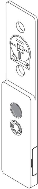
**ON/OFF (RTS26E5001B02):** If the window is opened, the Easywave code A (ON) is sent and if the window is closed the Easywave code B (OFF) is sent.
