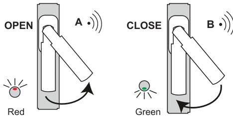
**OFF/ON (RTS26E5001B03):** If the window is opened, the Easywave code B (OFF) is sent and if the window is closed the Easywave code A (ON) is sent.
