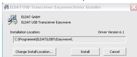
3. If required, define an alternative installation site at "Installation Location". Click on the button "Install" to install the drivers
